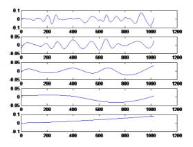
Fig. 2. Eemd decomposition of the outer ring fault signal
